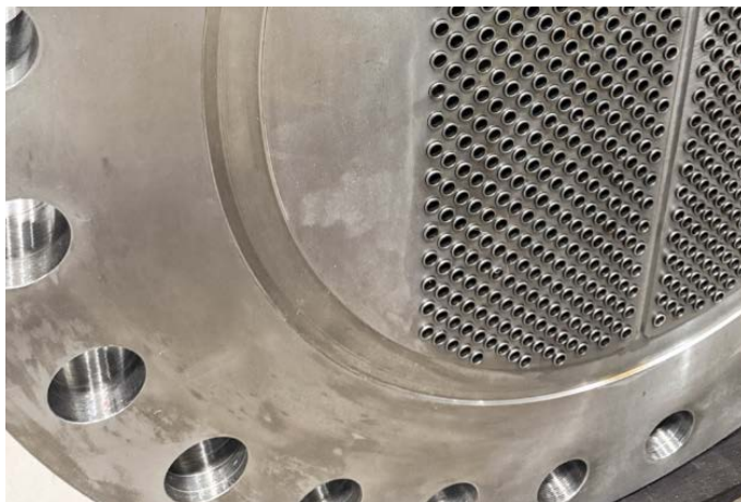
Figure 1. SA350 LF2 Tube Sheet, Image provided by SHECO - Southern Heat Exchanger
