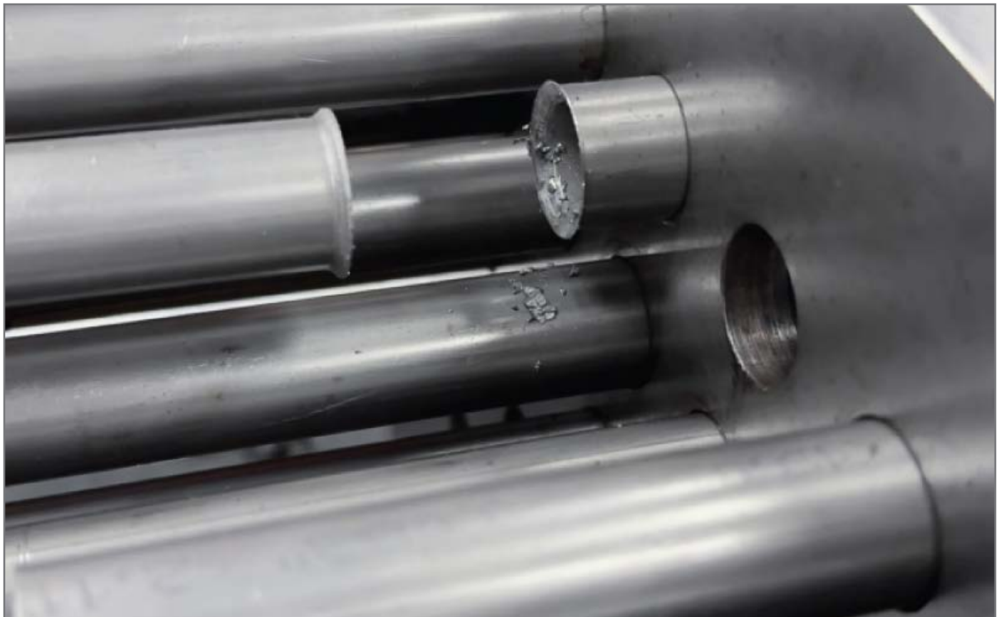
Figure 1. Example of failing to cut the tube on the opposite side behind the tube sheet
