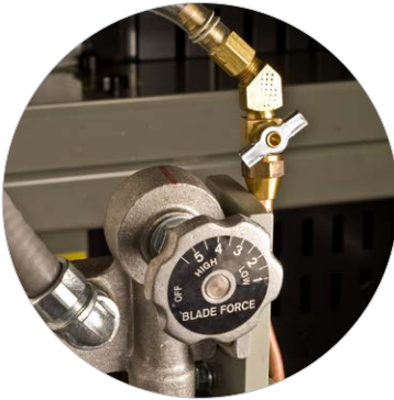
Automatic Cutting Force Control
