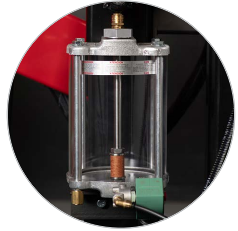
Automatic Tool Lubrication
