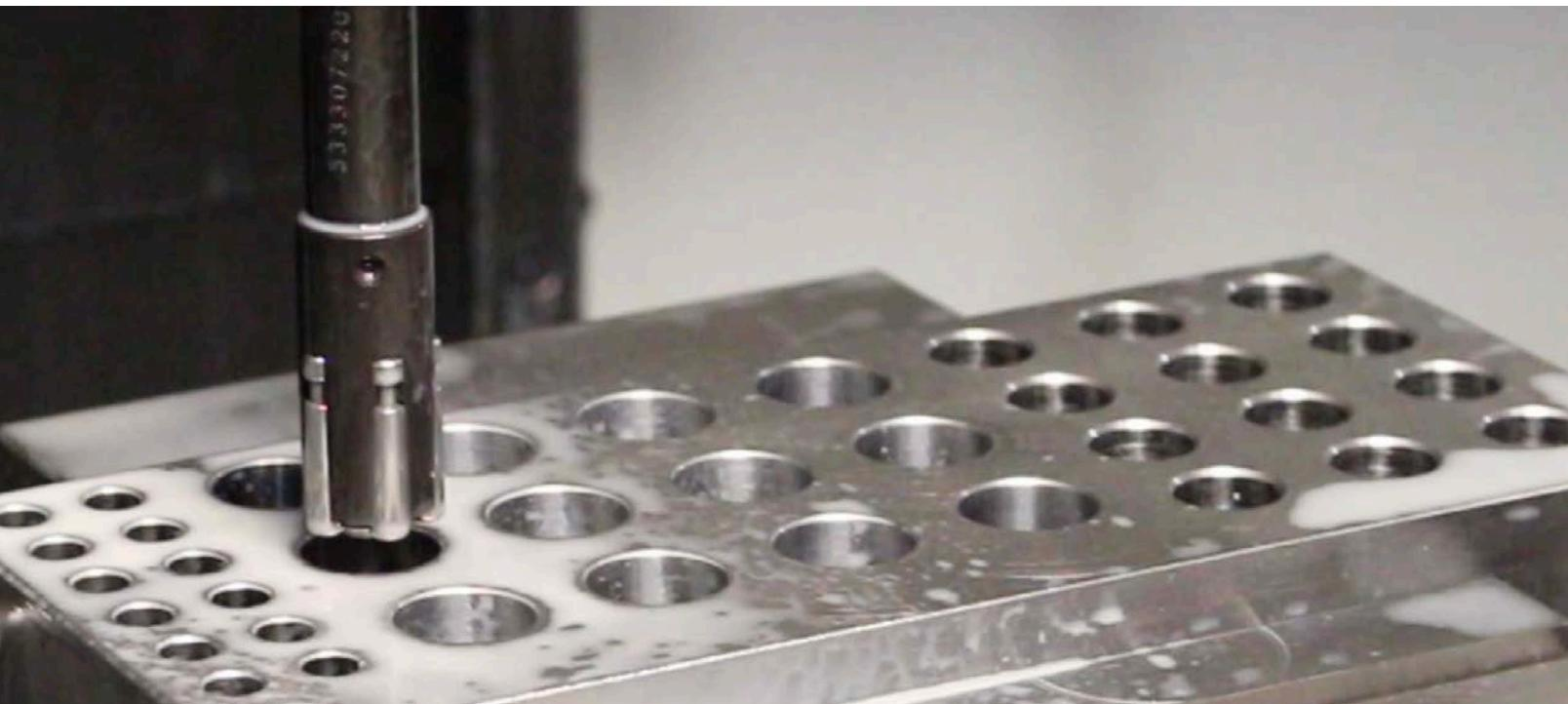
In addition to creating a smooth finish, burnishing also increases the material's resistance to wear by work hardening the surface of the workpiece. This results in better part life, as well as, better abrasion and in some cases corrosion resistance.
