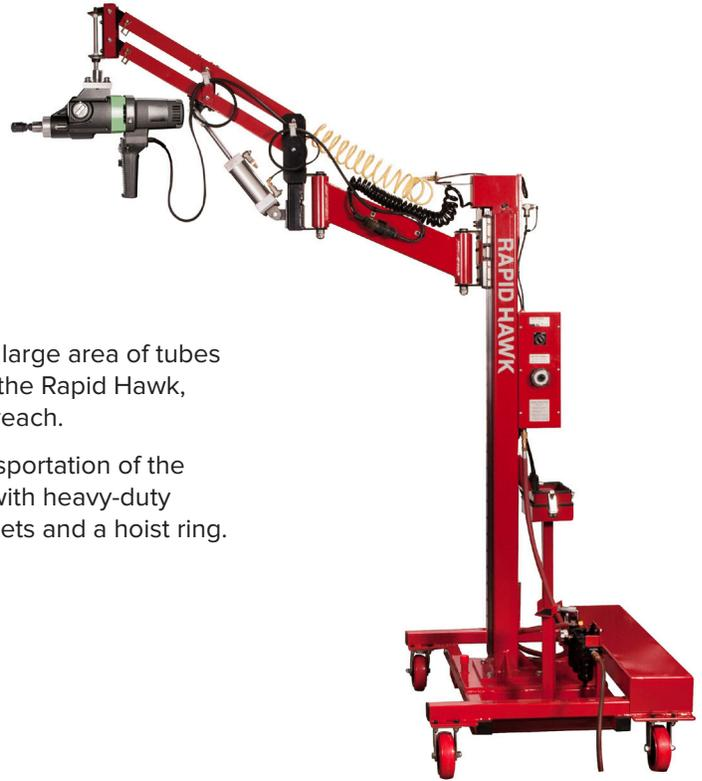
Ergonomically roll a large area of tubes without readjusting the Rapid Hawk, with its large radial reach.
